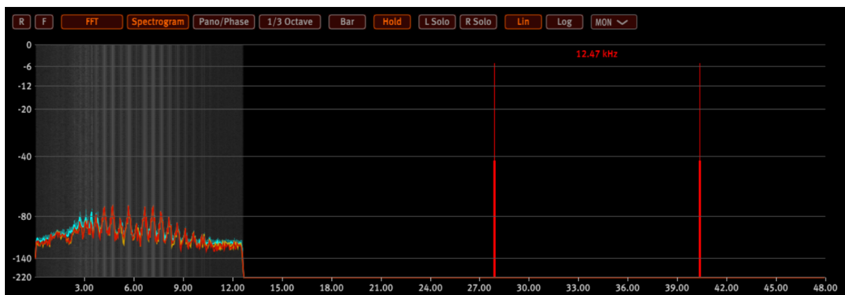
[27] Bandpass isolated distortion shifted into the audible frequency range
